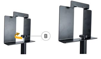
MOUNT THE MOUNTING PLATE WITH THE SCREW (B)
